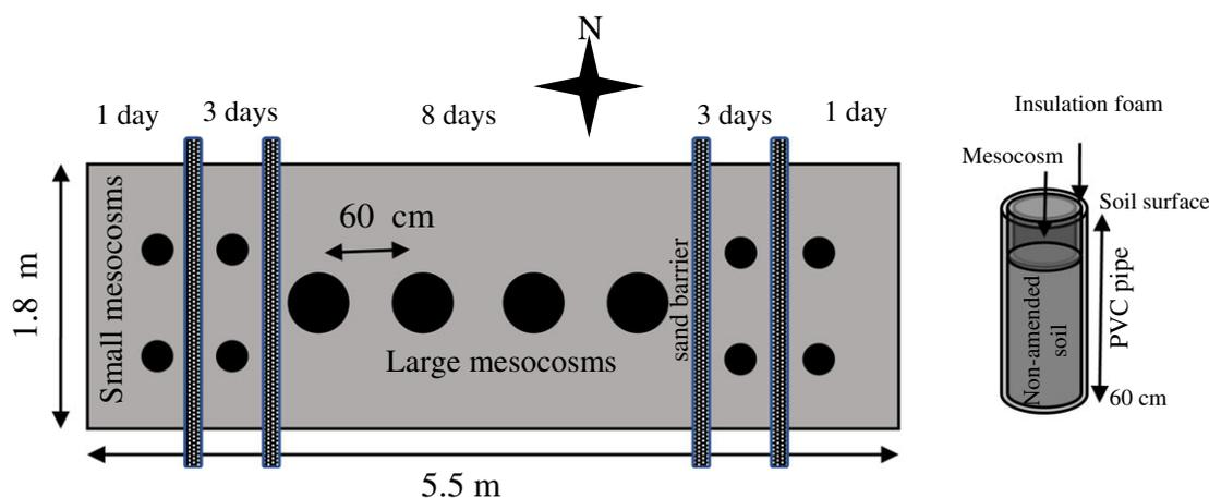
**Figure 1.** Schematics of the field plot and mesocosm arrangement (left) and of the PVC pipe with the mesocosms integrated (right).
