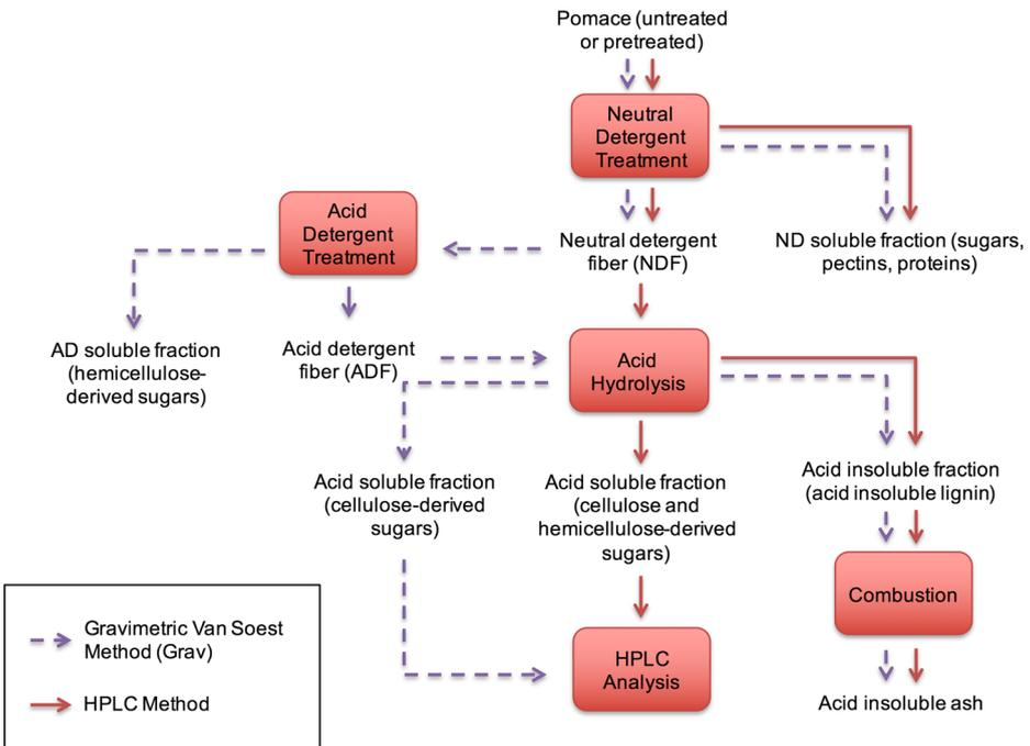
**Fig. 1** Flow diagram illustrating operations and material flows for the two analysis methods used to characterize pomace composition
