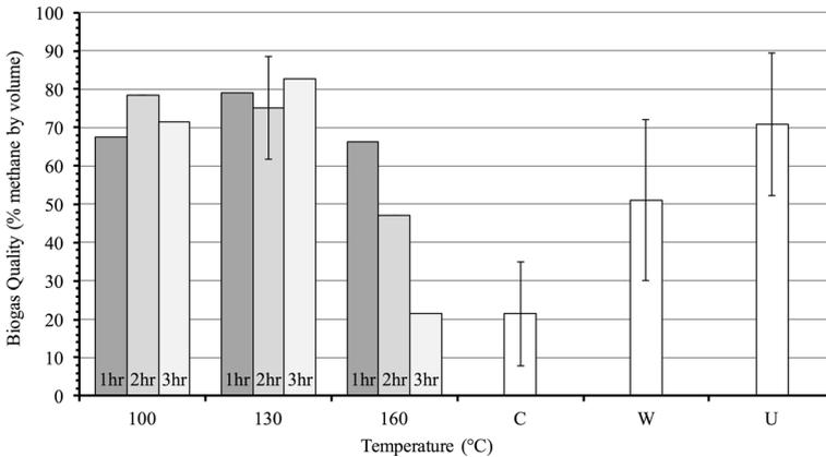
**Fig. 6** Mean biogas quality from anaerobic digestion of tomato pomace pretreated using various pretreatment times and temperatures. Pretreatment times are listed within bars. Biogas quality data is also provided for control samples containing no pomace (C), washed, non-pretreated pomace (W), and raw, untreated pomace (U). Error bars indicate one standard deviation. *n* = 5 for the center-point and *n* = 3 for the control treatments
