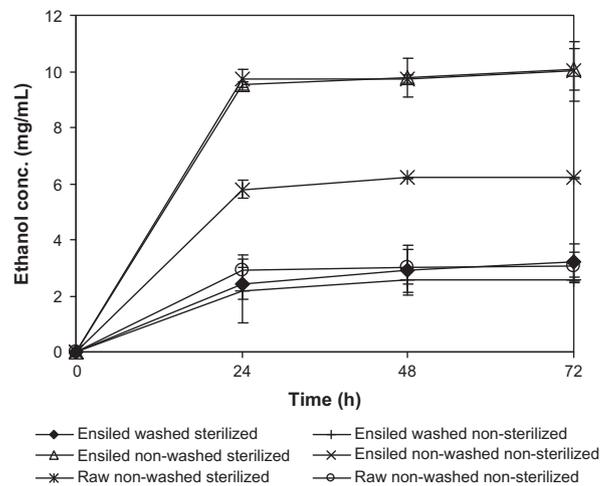
Fig. 5. Ensiled SBP fermentation by *E. coli* KO11 for ethanol production.
